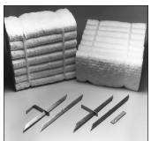
Bonded modules are typically mortared into place over existing refractory using .908 kg to 1.36 kg (2 to 3 lbs) of Fiberstick™ refractory cement per module. This lining over refractory (or veneering) approach not only increases the efficiency of the refractory lining but helps to protect it from further degradation.
